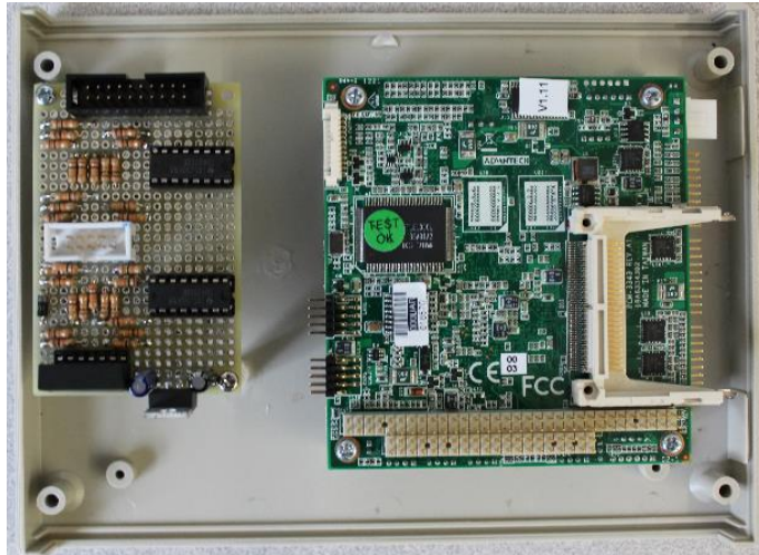
Figure 17. PCM-3343 SBC and Interface Circuit Mounted Inside the ABS Enclosure
