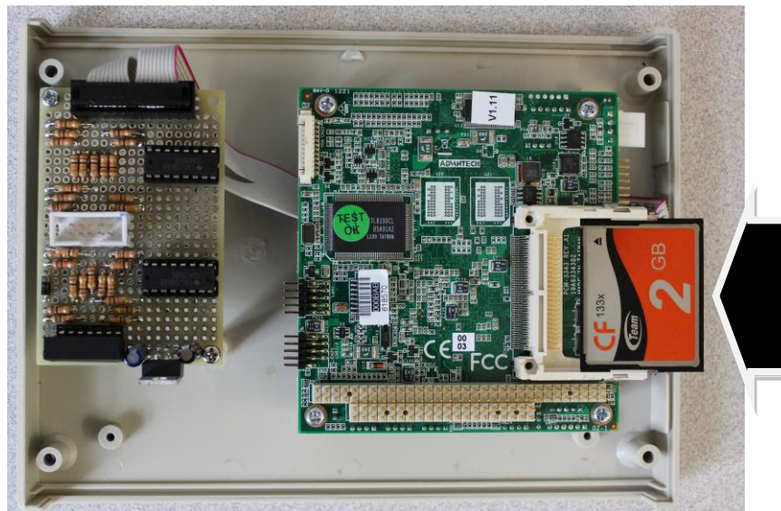
Figure 21. Mounting the CF Card
